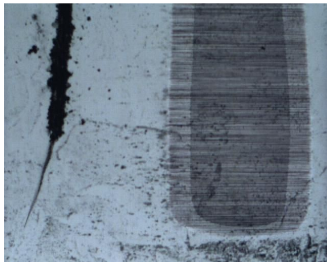
Figure 15. Junction depth (groove and stain) of control wafer 8 or more specifically the junction depth from the first diffusion (n-type).
