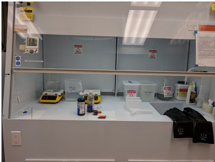
Cleaning, strip, and etching station
