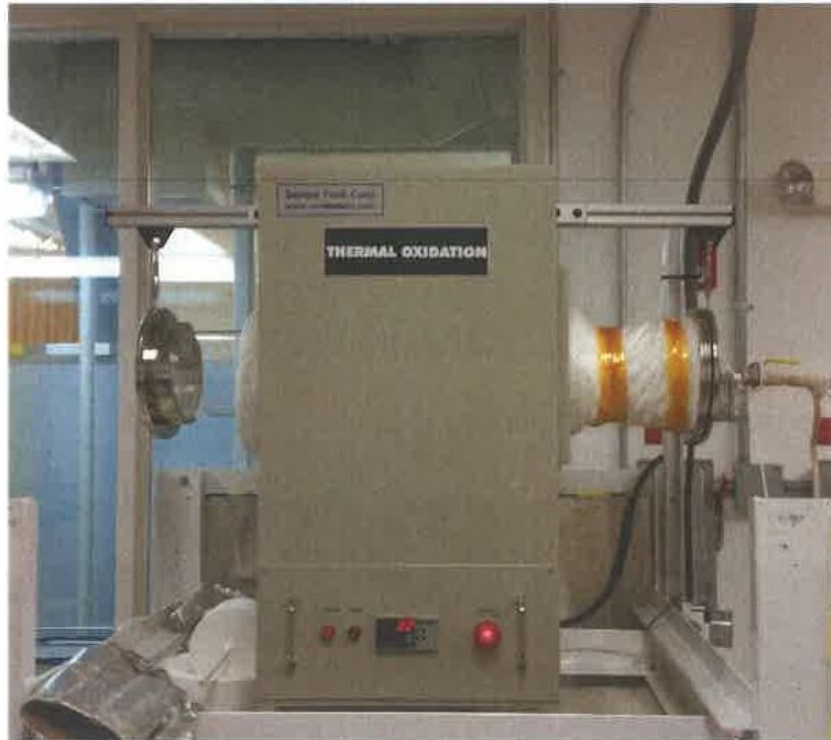
High temp furnace (oxidation and diffusion)
