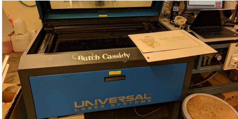
Figure 4. Universal Laser Systems laser cutter/engraver. This machine requires files to be in .dwg or .ai. The components must be scaled to be 1:1 in order to be printed correctly. This particular machine has a print area of 32" x 18". These could have been used to drill and make the holes if multiple passes were done.
